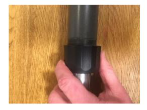
2. When the plastic sleeve is loose, move it and the blue sealing ring until you see the white plastic sleeve. Make a line at the white plastic sleeve according to the picture.
