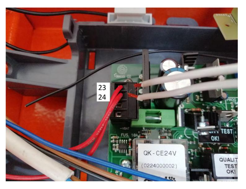
In the picture above you can see a close-up of the terminal block in which you need to connect the QK-LEDKITPCB cables. Please refer to the manual of QK-CE24V if you need help finding input pins n.23 and n.24. Setup completed. Now switch on the automatic barrier system and the LED tube will flash approximately every 0.8 seconds.
