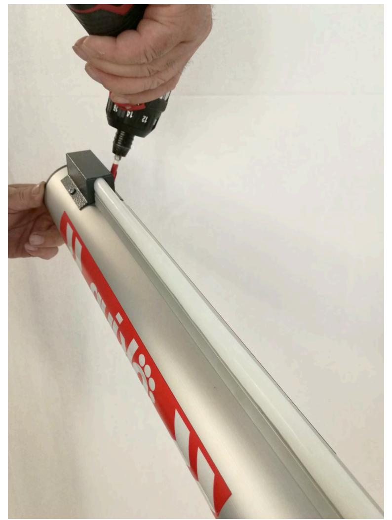
Take LED tube power supply cable and pass it through the apposite space so to reach the upper control board compartment
