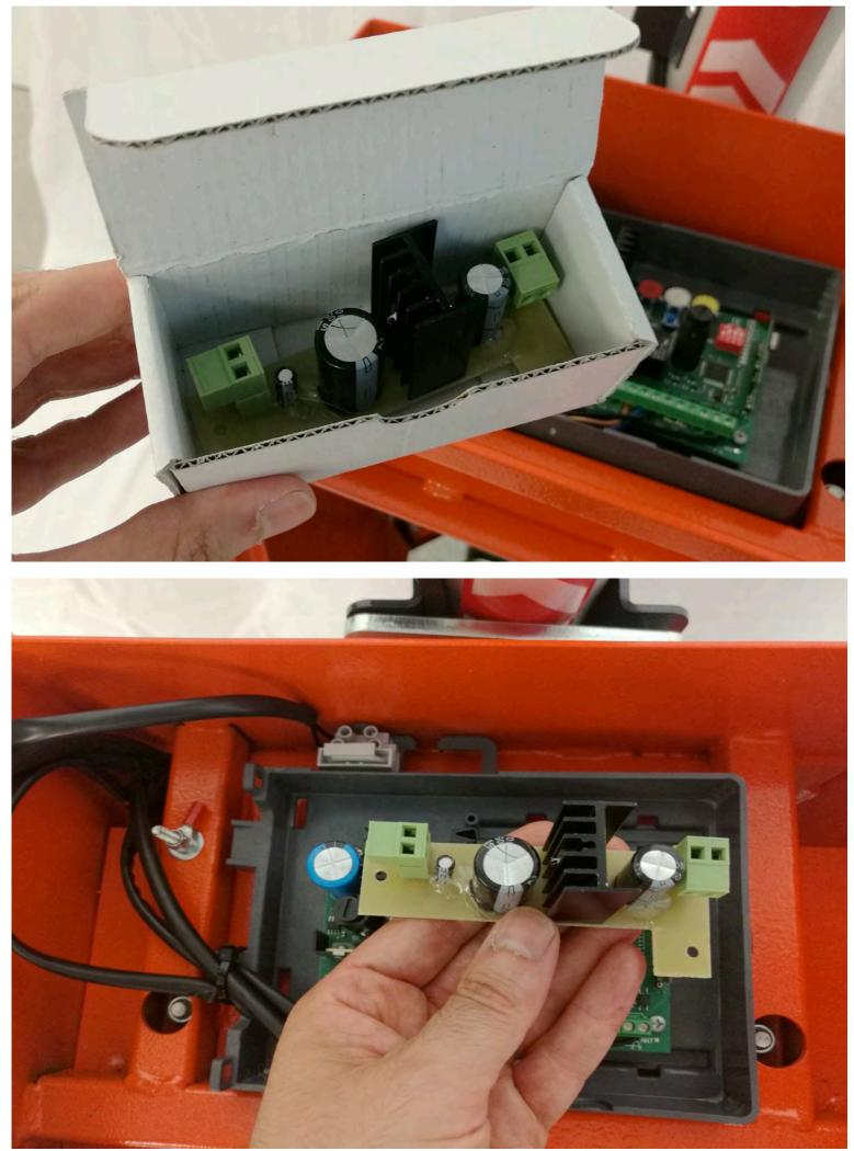
Connect LED tube power supply cable to apposite terminal block of QK-LEDKITPCB, respecting the polarity. Brown cable is (+), blue cable is (-).
