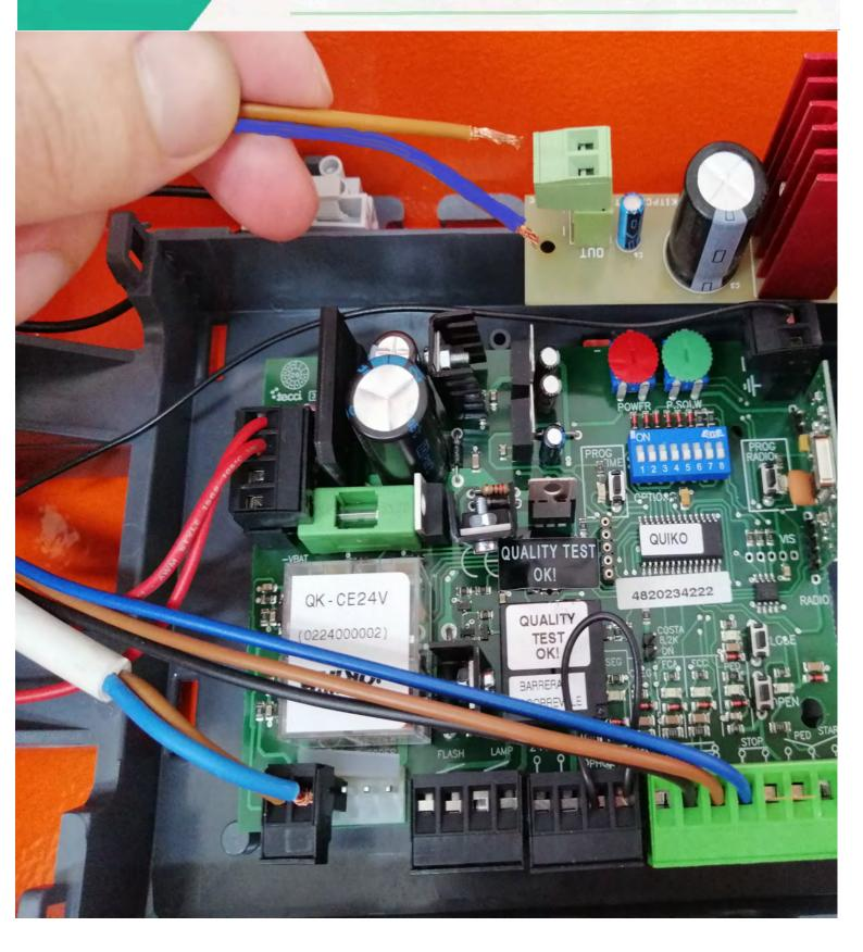
Connect two cables to the other terminal block of QK-LEDKITPCB and connect them to the 24V AC terminals n.23 and n.24 of the control board, as shown on the following pictures.
