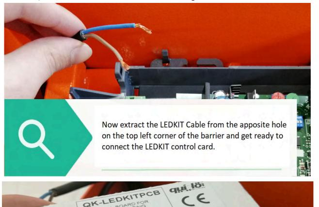
Take out LEDKITPCB from its box and connect the cables as shown on the next pages.
