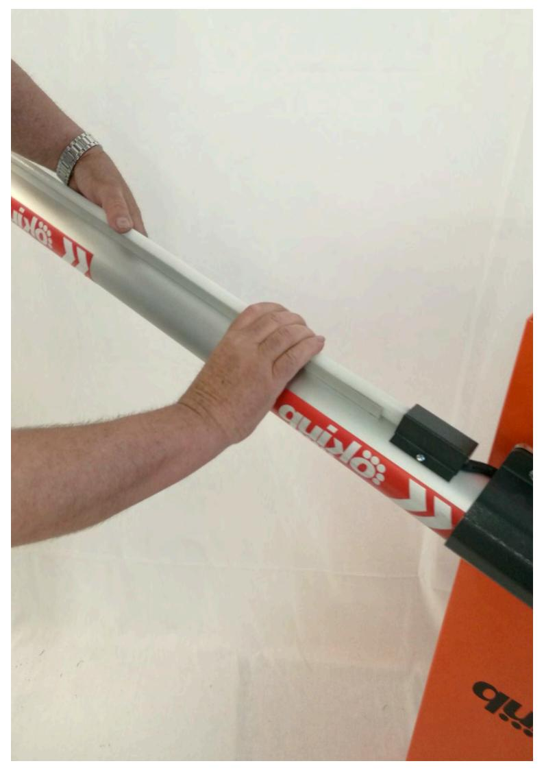
Place metal cover protection on last part of LED tube as shown on pictures
