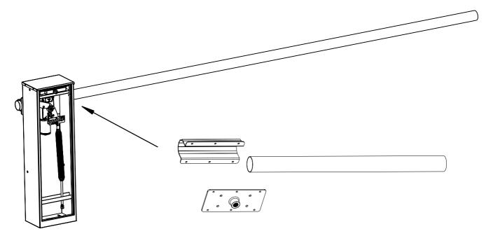
• Use the holes that are placed on the back of the barrier's body and on the boom plate support to pass the power supply cable (n.03) of the led tube. Cut a small hole in the black plastic cap of the hole to pass the cable through it, as shown in the picture.
