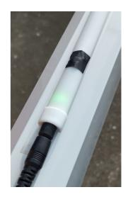
Connect the transformer to the power supply cable of the led tube and 230Vac power supply as per the below picture.
