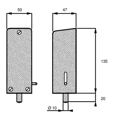
Power supply: 230 V 50 Hz Current absorbed: 0,15 A
