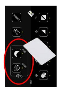
Once all the TAGs have been enabled, press ENTER or ESC to exit programming. Cancellation of enabled TAGs:
