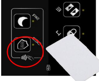
If the keypad lock is not yet activated: approach the TAG once and activate the keypad lock function (1 beep - the LED next to the icon lights up).
