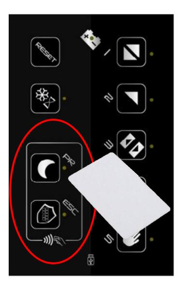
The area circled in red indicates the area in which to approach the Tag for use, <u>in any other area of the selector the</u> <u>TAG will not work</u>, the two icons indicate:
