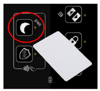
If the first opening is not yet activated: approach the TAG once and activate the first input function (1 beep - the LED next to the icon lights up).
