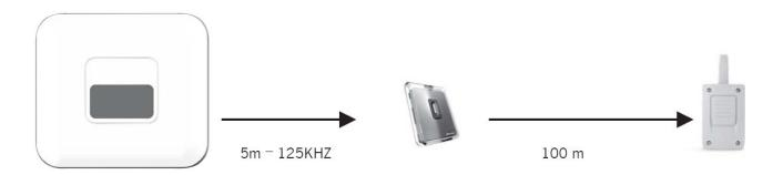
Once the equipment is supplied with electricity, the LED will flash for 3 times. By bringing the tag/transmitter close to the trigger antenna or pressing the button, the tag/transmitter will send a signal to the receiver in which it is programmed.
