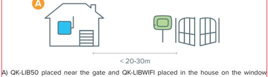
A) QK-LIB50 placed near the gate and QK-LIBWIFI placed in the house on the window closest to the gate. This solution allows you to open the gate both using Bluetooth and using Wi-Fi.
