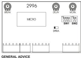
QK-CE220RLX is a control board used for automation of heavy duty sliding gates. Suitable for a connection with a clock (timer) which can be connected to the start single input for timely controlled openings / closings. QK-CE220RLX control board is in compliance with the following directives: EMC 2004/108/EC, BT 2006/95/EC and RADIO SETS 1999/05/EC.
