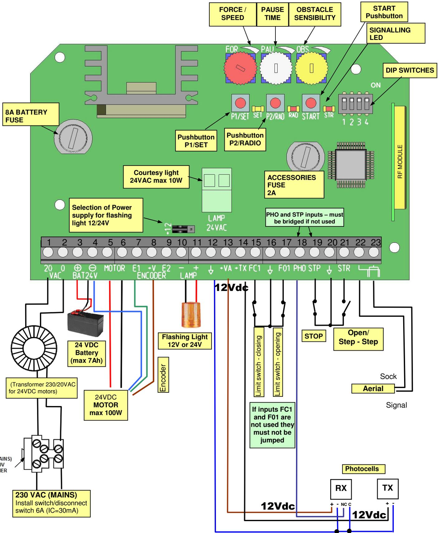
**NOTE:** The control unit is supplied with a trimmer to adjust the force of the motors set on maximum value (100%). Maintain this setting, which facilitates installation in difficult conditions (worn-out or not lubricated hinges, stress points etc.) Afterwards, reduce the force to obtain an operator movement that is slower and requires less force. **After having adjusted the force the learning procedure must be repeated.**
